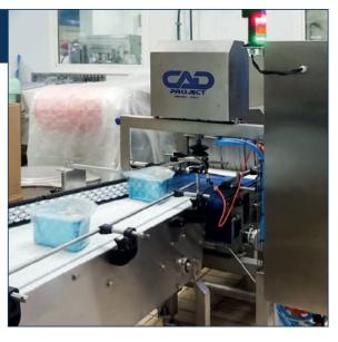
Manufacturing material: AISI304/316 stainless steel and blue POM-CProductPower supply:400V 3PH+N+G 50HzTraysPneumatic supply:6 bar
