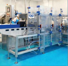
Manufacturing material: AISI304/316 stainless steel and blue POM-CPower supply:400V 3PH+N+T 50HzPneumatic supply:7 bar
