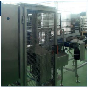
Manufacturing material: AISI304/316 stainless steel and blue POM-C Power supply: 400V 3PH + G 50 Hz Pneumatic supply: 6 bar
