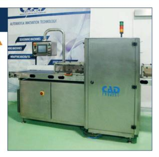
Manufacturing material: AISI304/316 stainless steel and blue POM-C Power supply: 400V 3PH+N+G 50Hz Pneumatic supply: 6 bar
