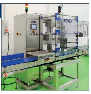
Manufacturing material: AISI304/316 stainless steel and blue POM-C Power supply: 400V 3PH+N+G 50Hz Pneumatic supply: 6 bar
