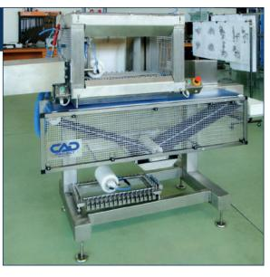
Manufacturing material: AISI304/316 stainless steel and blue POM-CPower supply:400V 3PH + T 50 HzPneumatic supply:6 bar
