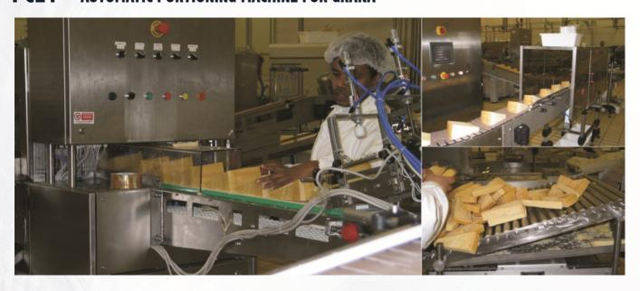
The machine cuts the big slices of grana into 2,3,4 portions and cuts the rind. The thickness is set by the operator panel.
